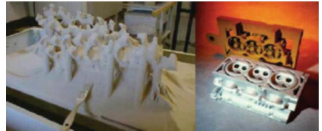
Fig. 14.12 Sand casting pattern for a cylinder head of a V6, 24-valve car engine ( left ) during loose powder removal and ( right ) pattern prepared for casting alongside a finished casting (Joint project between CAD/CAM Becker GmbH and VAW Südalumin GmbH, made on an EOSINT S laser-sintering machine, courtesy EOS)
