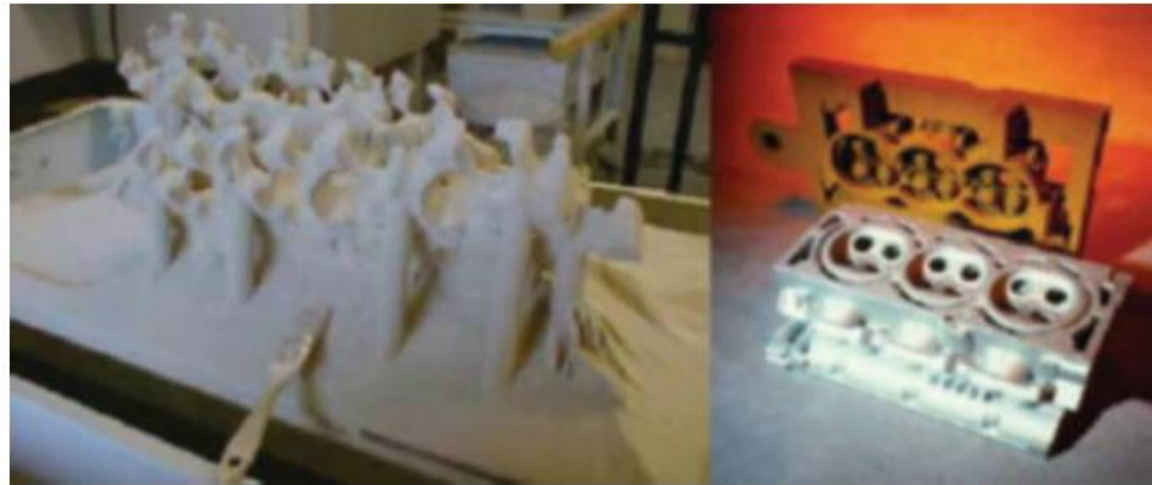
Sand casting pattern for a cylinder head of a V6, 24-valve car engine ( left ) during loose powder removal and ( right ) pattern prepared for casting alongside a finished casting (Joint project between CAD/CAM Becker GmbH and VAW Südalumin GmbH, made on an EOSINT S laser-sintering machine, courtesy EOS)
